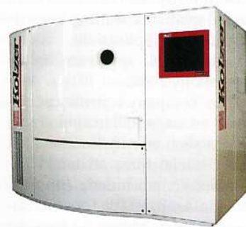
Kolzer sputtering system for metal deposition
