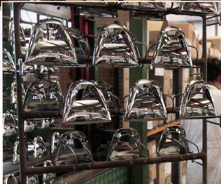
Above: Mounted on copper frames, mouldings await plating at Cromaplast Right: Examples of plated mouldings
