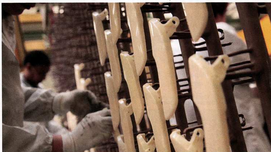
Above: Mounted on copper frames, mouldings await plating at Cromaplast Right: Examples of plated mouldings
